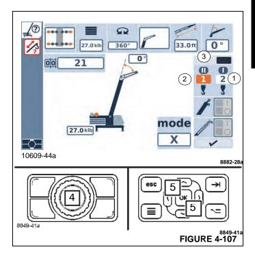
Position the slider bar (3, Figure 4-107) over the top of the hoist that is to be used. Example screen shot in Figure 4-107 shows the Auxiliary Hoist is selected.
