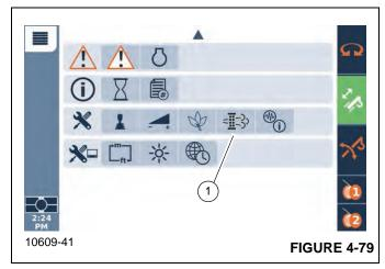
The Exhaust System Cleaning function screen (Figure 4-80) allows the operator to initiate or inhibit the exhaust system cleaning process.
