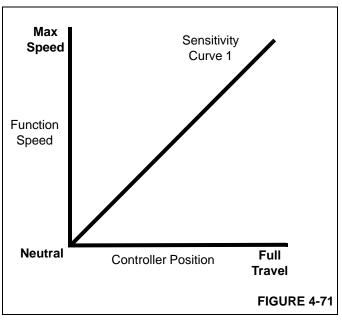
Selecting a sensitivity curve of 2 through 5 causes the function speed to be reduced, from the default sensitivity curve 1, relative to the same controller position over the full travel of the controller (Figure 4-72).
