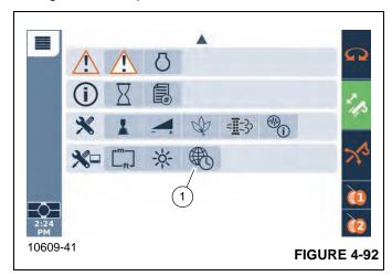
The Time Set function screen (Figure 4-93) allows the operator to set the time and the time format that is displayed on the ODM and RDM screens.
