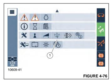
The Economy (ECO) Mode function offers the operator a convenient way to reduce noise and fuel consumption during craning operation. ECO Mode does this by automatically increasing the engine speed to an operator specified engine working speed when craning functions are operated and then decreasing the engine speed to idle speeds when no craning functions are operated.
