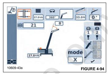
From the RCL Setup Screen, the operator can program the RCL either by entering a rigging code number from the *Load Chart Manual* or by entering the crane configuration using the setup wizard. The setup screen is also used to select the telescope mode, to include A, X, B, and M. Refer to the section titled *Telescoping the Boom*, page 4-23 for a description of the telescope modes.
