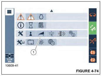
The Controller Speed function screen (Figure 4-75) allows the operator to adjust the crane function speeds relative to the position of the controllers. Adjustment is made as a percentage of full rated speed.
