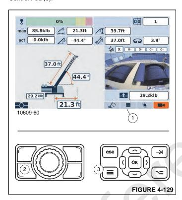
From the Menu Screen, select and confirm the Hoist Camera Icon (1, Figure 4-130) to open the full screen view of the hoist camera (2).
