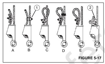
Of the methods shown, Grove prefers method A or F be used on Grove cranes, i.e., clipping a short piece of hoist rope to the dead-end or using a commercially available specialty clip (1) or wedge (2). It is recommended the dead-end tail length be a minimum of 6 rope diameters, but not less than 15.2 cm (6 in) for standard 6 to 8 strand ropes. For rotation resistant rope, the dead-end tail length must be a minimum of 20 rope diameters, but not less than 15.2 cm (6 in).
