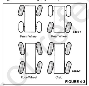
The Rear Steer Switch can only be operated when the speed of the crane is less than 8 km/h (5 mph).
