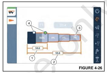
The Manual Telescope function screen shows an image that represents the boom (base section and the four telescope sections)
