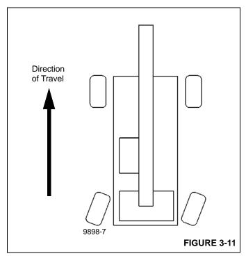
When rear wheels are not centered, the Rear Wheels Not Centered Alert in the Alerts Area (Figure 4-12) of the Operating Display Module (ODM) comes on (amber).
