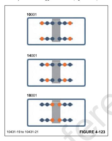
The standard MAXbase setups have at least two adjacent outrigger beams extended to 100%. The other two outrigger beams may be extended to 50% or 0% as shown in Figure 4-124.
