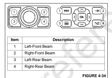
When a button at the Jog Dial or Navigation Control Pad is pushed and held, the corresponding O/R beam image turns orange to indicate that it is actively moving. An arrow will appear to indicate whether the beam is extending or retracting. In the following example (Figure 4-35), the top image shows the Left-Front O/R beam is extending and the bottom image shows the Left-Front O/R beam is retracting.
