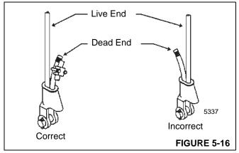
4. Insert hoist rope end in socket, form a loop in the rope, and route rope back through socket allowing the "dead" end to protrude from the socket. Make sure dead end of the rope is long enough to apply end treatment after wedge is seated.
