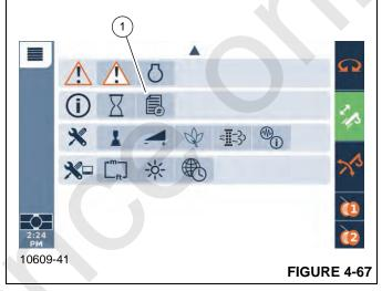
The Software Versions function screen shows the current software versions for all of the software installed on the crane.
