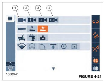
These camera view function icons are used to select which camera view is displayed on the Camera View Screen (Figure 4-23).
